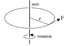
Imagine a force of F Newtons acting tangentially at a radius of r metres
